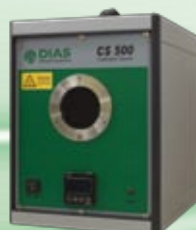
PYROTHERM CS 500 Temperature range: 50 °C to 500 °C
